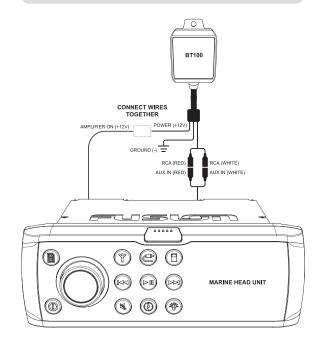
FUSION recommends that the MS-BT100 is mounted in an elevated position as far away from metal work as possible. This will ensure maximum range for Bluetooth audio streaming. Any barrier between the MS-BT100 and your streaming device will reduce the range.
