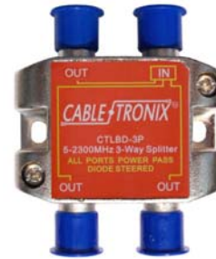
CTLBD-3P 3 Way Splitter All Legs Power Pass
