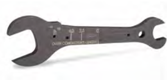
CT-7812 Combination Tool (open end wrench for connector body, chamfer tool, file, inner conductor gauge, jacket cut-off gauge) for 1/2 in and 7/8 in coaxial cable
